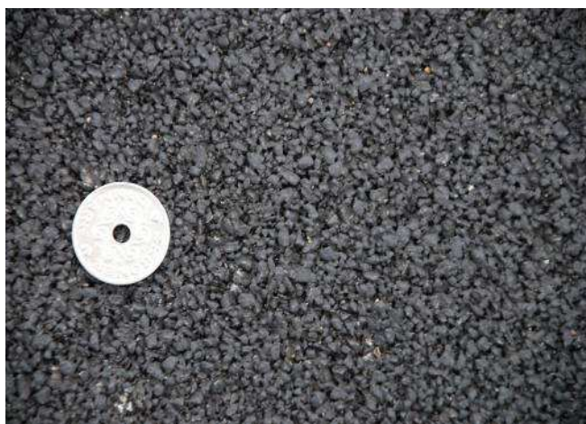
Rys. 9.12. Nawierzchnia jednowarstwowa (DVS-DRI Super Quiet Traffic International search for pavement providing 10 dB noise reduction, Danish Road Institute Report nr 178, 2009)
